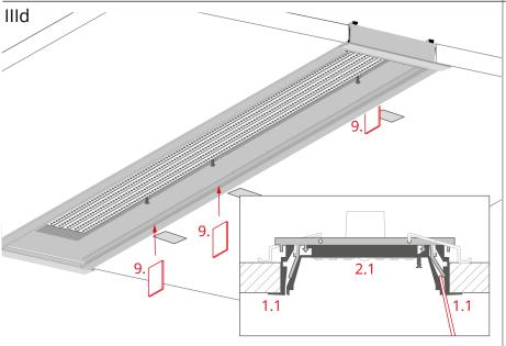
To prevent the OMODO-100 profile from falling out, insert wedges temporarily (9). They should be inserted into the marked spots in the gap between item (1.1) and item (2.1). There should be one wedge for each marked element (1.2) and they should be placed from the side of the profiled orientation line.
