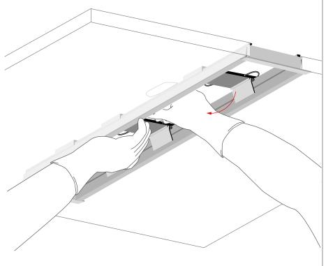
Lock the springs (1.4) at each item (1.2) by turning them, pressing them against the plate surface and sliding under the edge of the item (1.2) as shown in the figure.
