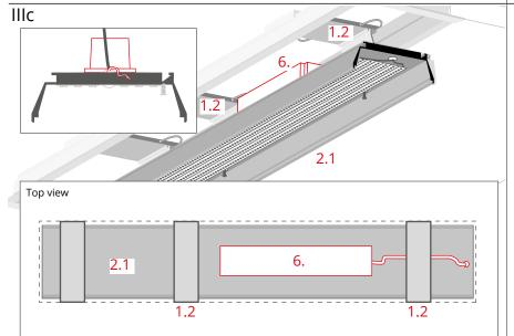
Mount the power supply (6) on the back of the profile in such a position that it fits into the opening of the RAM-KOL-100 profile.
