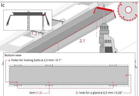
a. Drill holes for locking bolts in the profiled orientation line in the profile (2.1).
