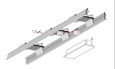
If the power supply (6) does not fit into the openings of the RAM-KOL-100 profile, its items (1.2) must be slid further apart accordingly.
