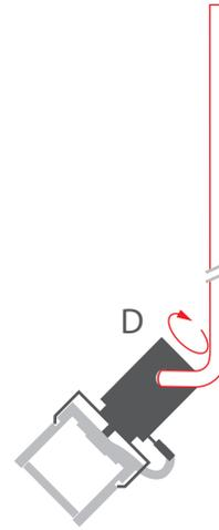
**3. NOTE!** The position of the lighting fixture on the arm can be adjusted in the range of 360° (depending on the distance of the fastener from the edge of the extrusion).
