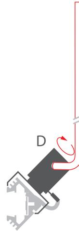
**3. NOTE!** The position of the lighting fixture on the arm can be adjusted in the range of 360° (depending on the distance of the fastener from the edge of the extrusion).
